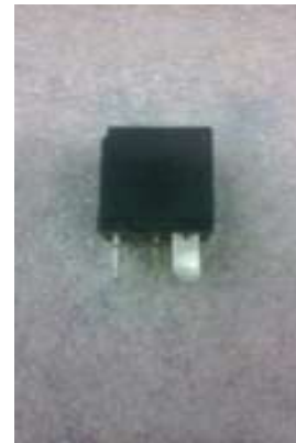
Controller Relay AA01-0016
