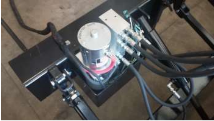
Figure 7 Hydraulic Wings Pump Above Fixed Wing Pump On Right
