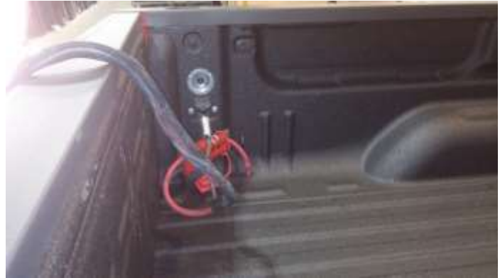
Figure 6 Typical Remote Switch Mounting, Shown On GM Pick-up Installation
