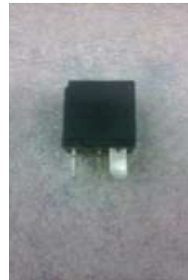
Controller Relay AA01-0016
