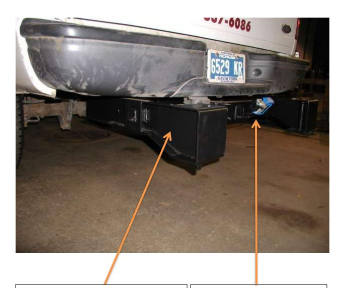
QD Arms Attached Into Side Of Hitch Tube, QD Channel Attached To Arms Using Long Vertical QD Pins Electrical Connections Under OEM Bumper
