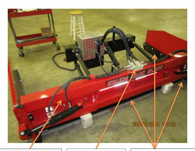
2014 Models Had Slide On Moldboard Ends. This Is The Case For Hydraulic & Fixed Wings **2014 Had Removable Bulkhead Fitting Plate**
