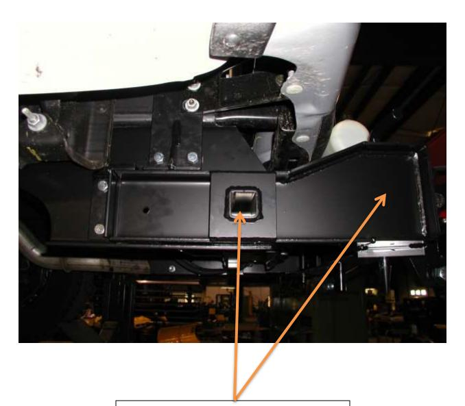
QD Arms Attached Into Side Of Hitch Tube, QD Channel Attached To Arms Using Long Vertical QD Pins
