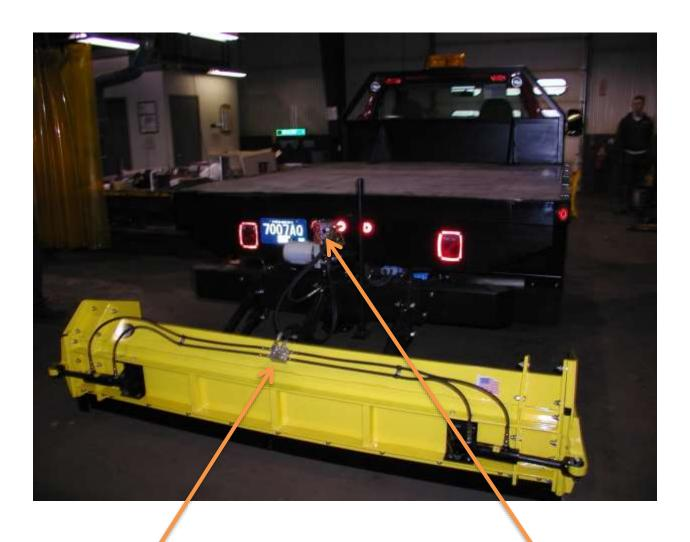
Originally the hydraulic wing models had cylinders working together instead of separate controls
