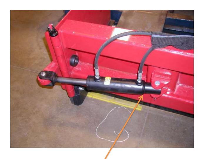
Non Adjustable Wing Cylinders New Adjustable Cylinders Are Compatible
